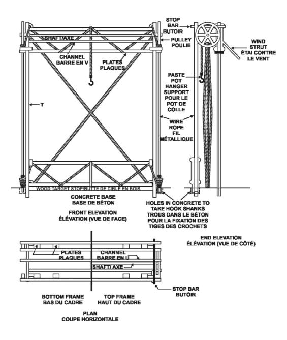
Figure 2 - A plan of the Hythe pattern target frame, taken from a Canadian bilingual manual (Candian National Defence, 'Range Construction and Maintenance, B-GL-381-002/TS-000, dated 2009)
